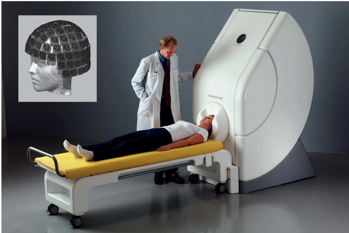
Figure 2 An example of a state-of-the-art MEG system. Although not apparent, this system is housed in a large shielded room. The entire structure at the subject's head is called a gantry, and it is set to perform an MEG scan of a subject in the supine position. The gantry can also be swung upward when needed to accommodate a subject in the sitting position. As in Figure 1 , the subject wears no magnetic material. The subject's head is shown positioned in a helmet-shaped liquid helium dewar, as part of the gantry. This dewar contains 306 sensors surrounding the head, illustrated in the inset at left, oriented as if the patient was in the sitting position (head vertical). The sensors consist of 306 'pickup coils' centered at 102 locations over the head, with three different coils at each location. One coil is a simple outside square and hence a magnetometer; the other two are rectangular planar gradiometers, oriented at right angles to each other. Three SQUIDS are part of each square. Thus, the entire system consists of 102 magnetometers and 204 planar gradiometers for a total of 306 MEG channels. This MEG system, called Vector View 306, is made by Elekta AB (Finland). Other manufacturers supply similar systems, each with its own distinctive features.
